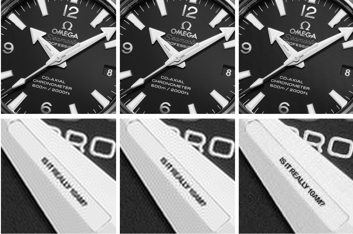
Figure 24: Subsampling a fixed number of 512^2 = 262144 Fourier coefficients. Left : 2048 \times 2048 linear reconstruction from the first 512^2 = 262144 Fourier coefficients (zero padded). Middle : 2048 \times 2048 reconstruction in the DB8 basis via \ell^1 -optimization from the first 512^2 = 262144 Fourier coefficients (zero padded). Right : 2048 \times 2048 reconstruction in the DB8 basis via \ell^1 -optimization from the same number 512^2 = 262144 of Fourier coefficients taken from a multi-level scheme consisting of 100 levels, as used in Figure 22.
